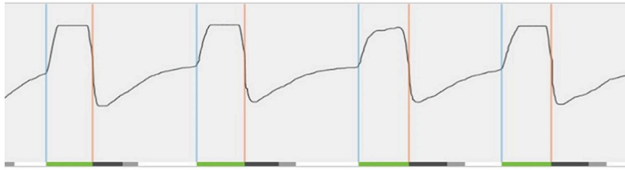
FIGURE 5 | Real-time sensor waveform test during implantation. The respiration and stimulation are shown in the graph. During breathing, a change in pressure is detected by the sensor. This information is sent to the implantable pulse generator. Stimulation (green line at bottom) is triggered (blue vertical line) and should last until expiration is detected (orange vertical line). In order to prevent stimulation immediately after exhalation, the off period begins (dark gray line at bottom). After the off period, a new stimulation can be triggered. When this does not occur immediately, there is a period without stimulation (light gray line at bottom).
