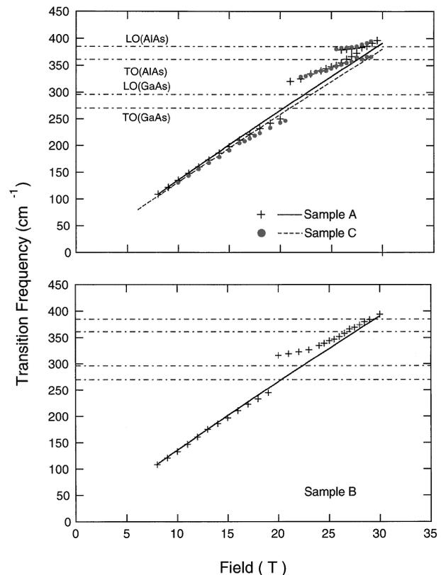
FIG. 1. Experimental data for all three samples. The tilted straight lines in the figures are the calculated CR transitions including nonparabolicity only.
