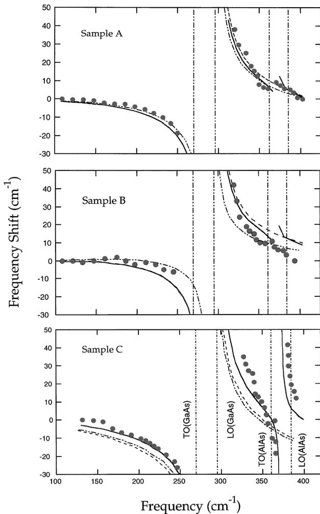
FIG. 3. Plot of frequency shift vs frequency for three samples. The dots are experimental data. The dashed curves are for coupling with only bulk GaAs optical phonons, the dash-dotted curves include screening effects within the RPA in addition to the coupling with the GaAs bulk phonons, and the solid curves consider the effects of IO phonon and slab LO optical phonon modes.
