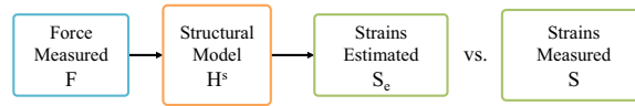
Figure 8: The estimated strains are calculated based on the structural model and a measured force.
