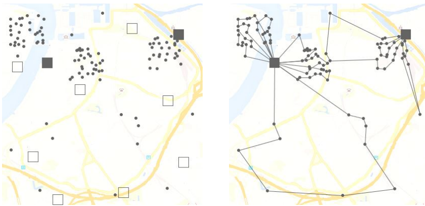
Figure 7.1: Decomposition of an LRP. We first generate location options (left), and evaluate each location option by solving the respective MDVRP (right). The example is taken from instance ‘112112’ by Tuzun and Burke (1999).
