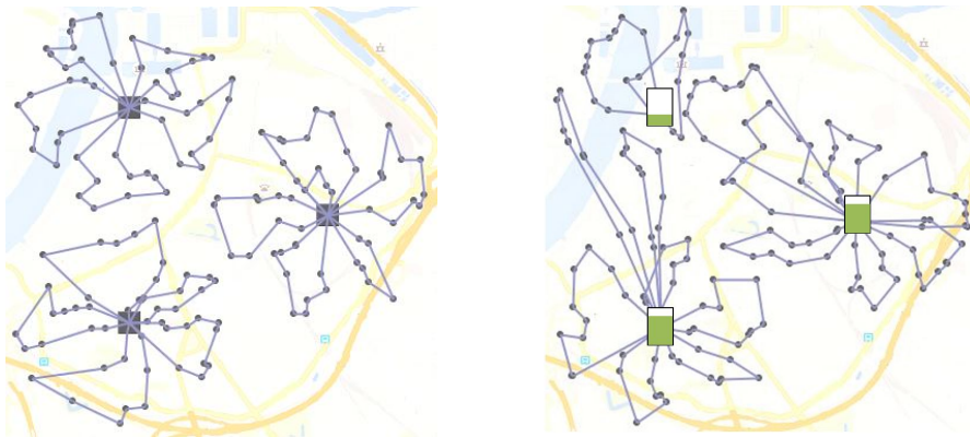
Figure 6.2: Routing solutions in a multi-depot context can be computed in different ways. (Left) Each depot only delivers customers in ‘its area’. (Right) Each depot can deliver any customer as in classical MDVRPs. If we consider the inventory levels as constraint in MDVRPI, we might arrive at a slightly worse routing.
