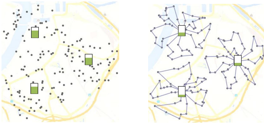
Figure 6.1: Integration of inventory management and routing. A company with several depots has to plan the inventory in the depots, as well as to plan delivery routes to fulfill customers' demand.
