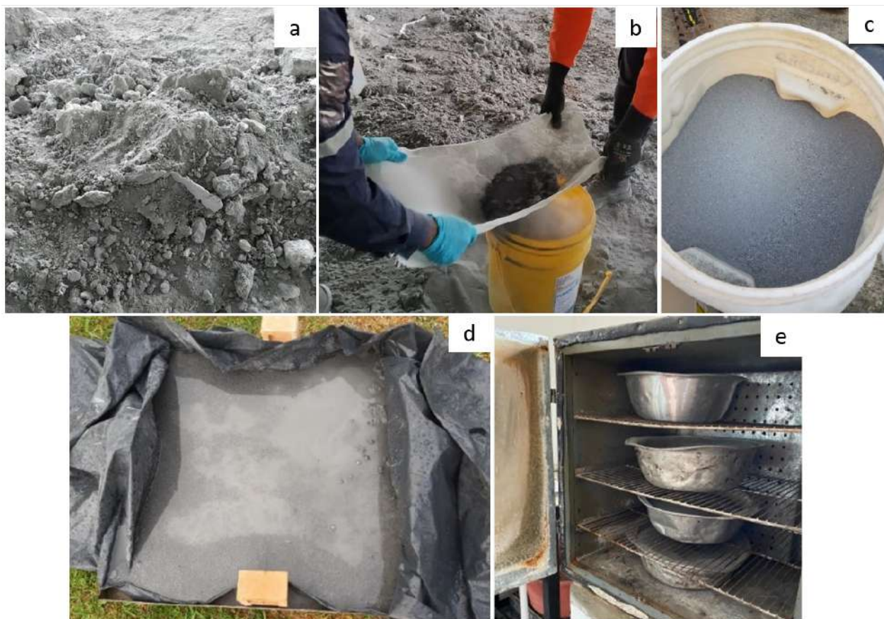
Figure 2. (a) AD at the collection site, (b) initial sieve, (c) AD, (d) washing process, and (e) drying process.
