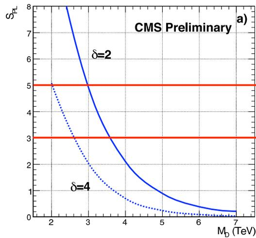
Fig. 11. Sensitivity for a  $5\sigma$  discovery of monojet events in CMS as function of the mass  $M_D$ , for 2 and 4 extra dimensions  $\delta$ , for an integrated luminosity of  $0.1 \text{ fb}^{-1}$ .
