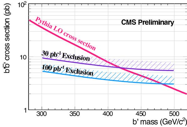
Fig. 10. 95% C.L. exclusion limits for the detection of heavy  $b'$  quarks in the  $tW$  decay, for 30 and 100  $\text{pb}^{-1}$  of integrated luminosity.
