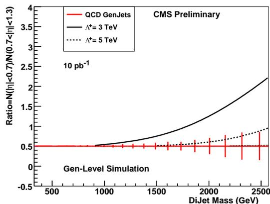
Fig. 2. Ratio of central to forward di-jet events as function of the di-jet invariant mass. The curves show the QCD prediction as well as the prediction for contact interactions for two scales. The error bars show the sensitivity for  $10 \text{ pb}^{-1}$ .
