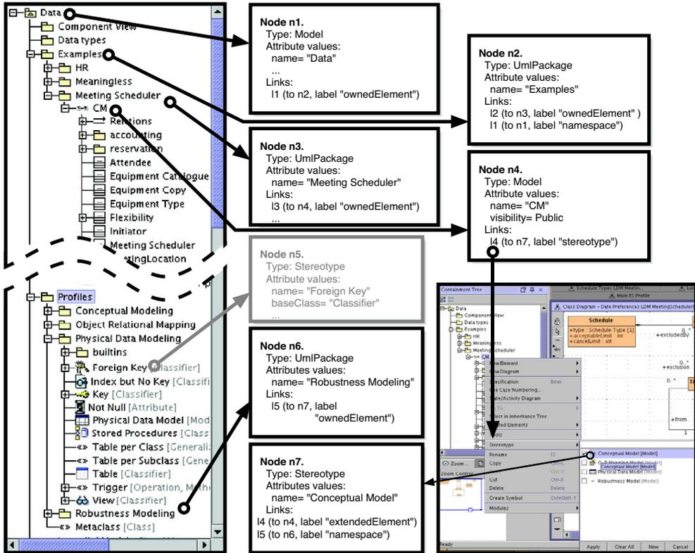
Figure 3. Relation between the UML editor and the underlying model graph.
