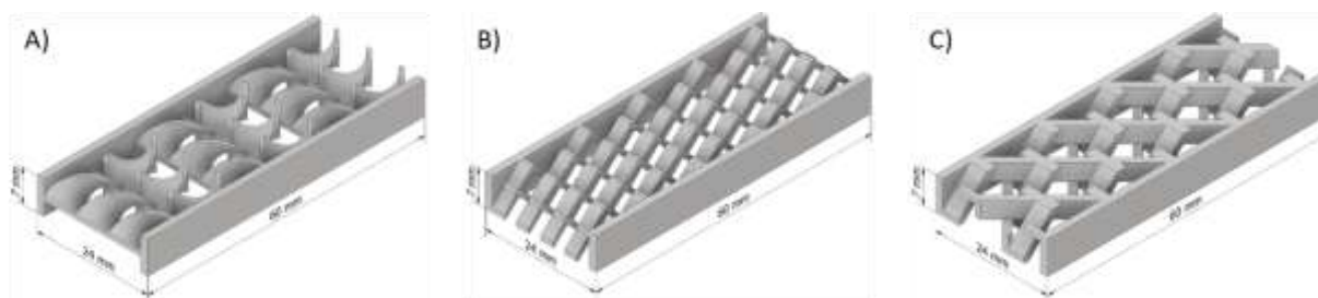
Fig. 2: Classes of the structured 3D electrodes: (A) Kenics electrode, (B) RLPD electrode and (C) SMX electrode.
