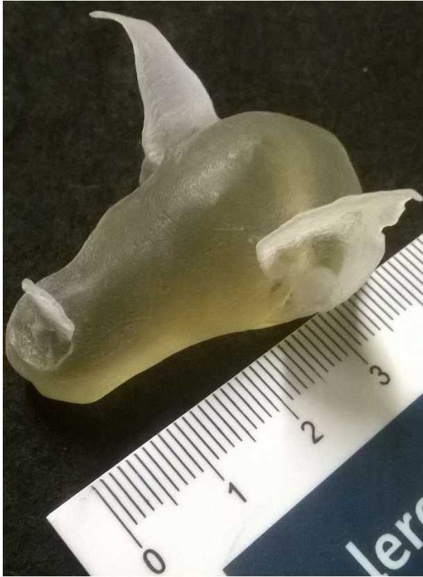
Figure S1: Photo of the plastic replica of a Phyllostomus discolor head. The replica (scale 1:1) was used for the echo-intensity measurements in the flight tunnel. During the measurements a Knowles FG series microphone (FG-23629-D65) was positioned in the left ear at the entrance of the ear canal (not shown here).
