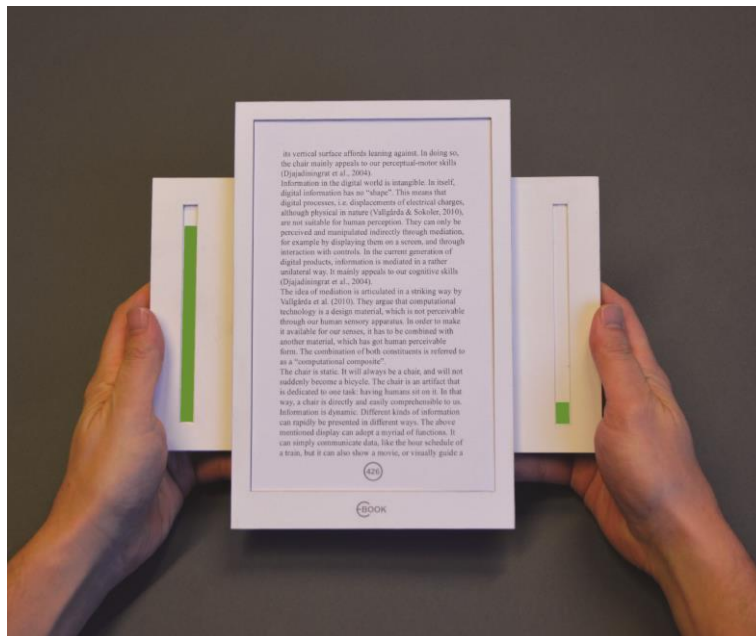
Fig. 25 The device in reading mode, at nine tenth of the total amount of pages
