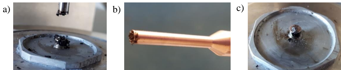
Figure 8. Photograph of both plates after the strain sweep: a) The sample after the test; b) The upper plate; c) the bottom plate
