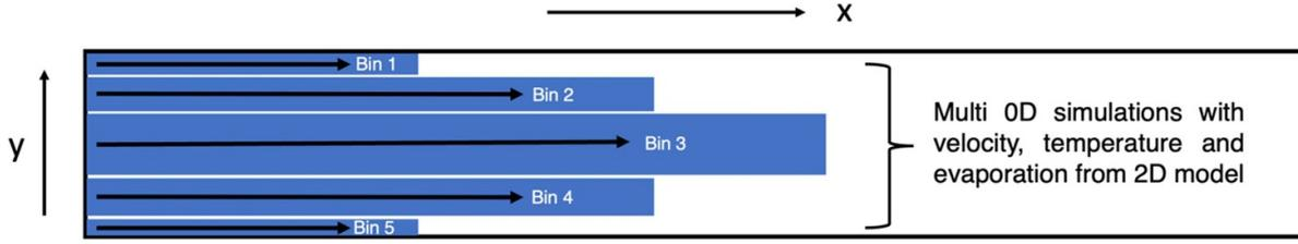
**Figure 3.** The channel is separated in different bins. The chemical kinetics of each bin is solved by a different 0D model with different parameters, such as gas velocity, gas temperature and water vapour concentration. For simplicity only 5 bins are illustrated while for the model, 11 bins are used.
