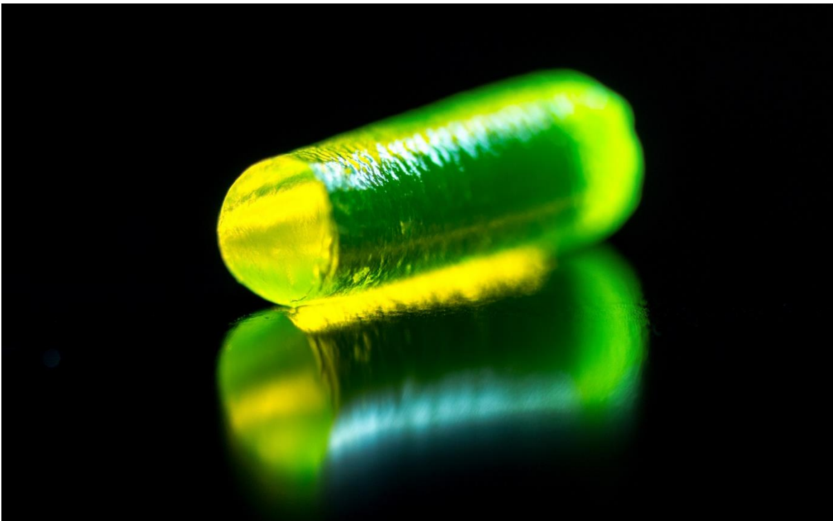
Fig. 10. Extruded insert loaded with sodium fluorescein. The dimensions of the inserts are 2 mm diameter and 10 mm in length.
