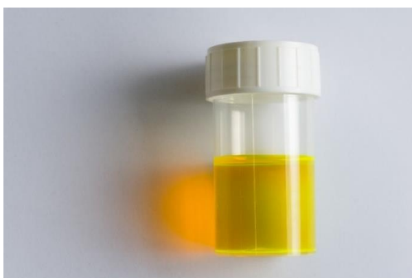
Fig. 9b. End result after a polymer cylinder had been fully submerged in a sodium fluorescein solution over the course of six weeks. Notice how the highly viscous mass does not appear to flow when lying flat on the surface. Picture taken from above. The samples in these pictures have only been prepared and photographed for demonstrative purposes.
