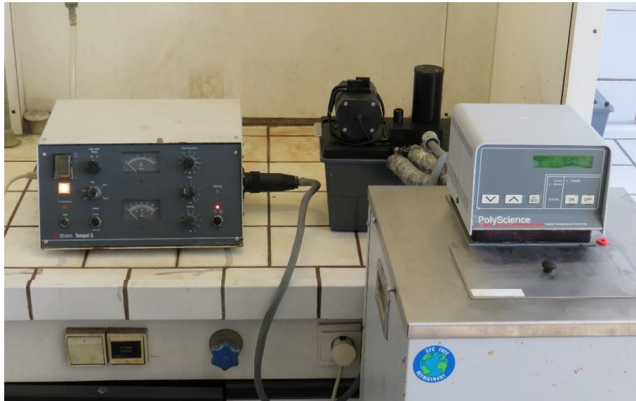
Figure 3–5 The Struers TenuPol apparatus used in this work (control panel, electroplating cell and tank, and the cooling system).
