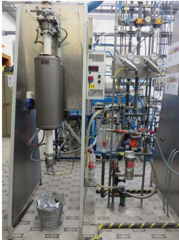
Figure 3–1 The vertical furnace used for heat treatment.
