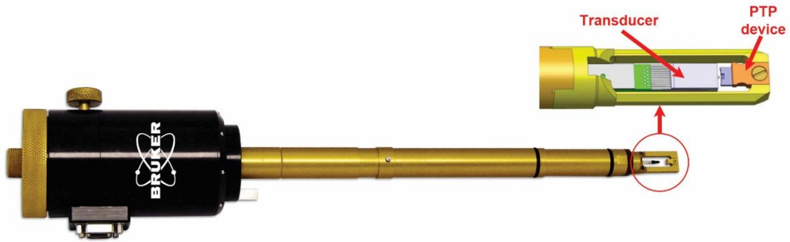
Figure 3–11 A Hysitron PI 95 TEM Picoindenter with PTP device installed.
