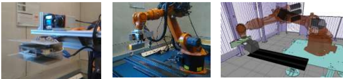
Fig. 2. Dynamic line scan setup using an industrial robot arm and its corresponding simulation environment.
