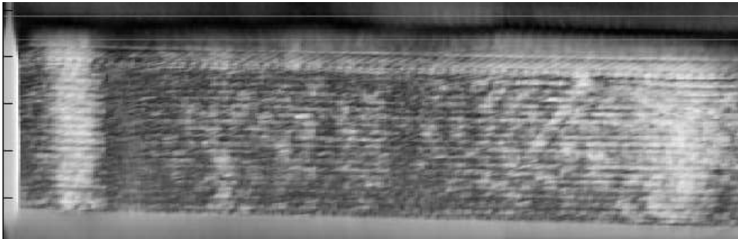
Fig. 15: Stiffener D, 2000 W/m power, translation speed of 5 mm/sec, 3 Hz, Correlation
