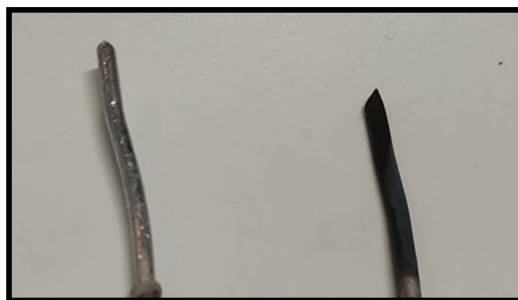
Figure 7.18. Sn working electrode after 1 h electrolysis in KHCO 3 2 M in presence of 20 mM of [Zn(cyclen)] 2+ (left) and 2 mM of [Zn(imidazole) 3 ] 2+ (right).
