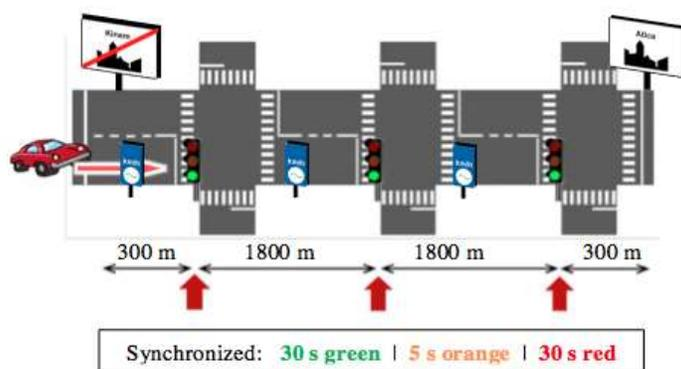
FIGURE 1 The challenge of the *Green Wave* learning module: Build and program a car so that it can pass three synchronized traffic lights when they are lit green, on a scale model of the depicted situation
