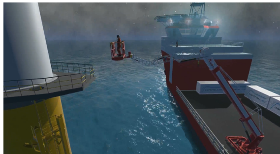
Figure 3.6: 3D real-time simulation of a motion compensated crane. Taken from [97].
