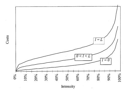
Figure 2: Operating costs at different levels of age and intensity of utilization
