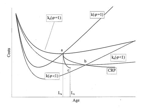
Figure 1: The single-machine model
