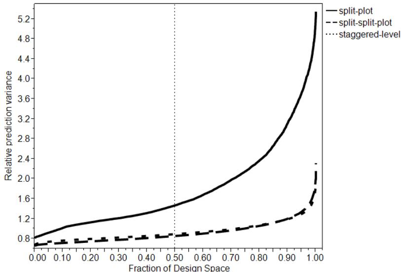
**Figure 1:** Fraction of Design Space (FDS) plot for the 28-run I-optimal split-plot, split-split-plot and staggered-level designs, constructed assuming  $\eta_\delta = 1$  and  $\eta_\gamma = 1$ .
