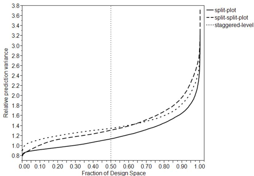
**Figure 2:** Fraction of Design Space (FDS) plot for the 20-run I-optimal split-plot, split-split-plot and staggered-level designs, constructed assuming  $\eta_\delta = 1$  and  $\eta_\gamma = 1$ .
