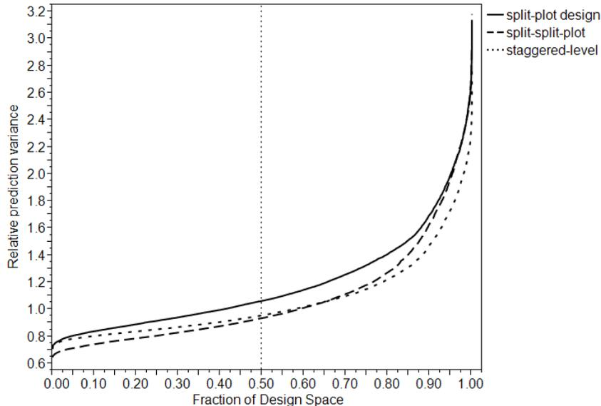
**Figure 3:** Fraction of Design Space (FDS) plot for the 36-run I-optimal split-plot, split-split-plot and staggered-level designs, constructed assuming  $\eta_\delta = 1$  and  $\eta_\gamma = 1$ .
