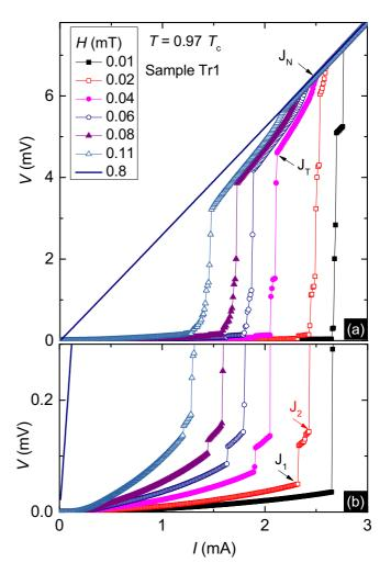
FIG. 2. (Color online) (a) Experimental current-voltage characteristics for sample Tr1 obtained at  $T=0.97T_c$  and for several applied magnetic fields. The magnetic field  $H=0.8~\rm mT$  is above the upper critical field and the curve corresponds to the Ohmic response in the normal state. (b) Zoom-in of the low-voltage regime. The onset of different dynamic phases is indicated by arrows.
