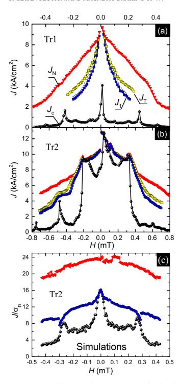
FIG. 4. (Color online) Dynamic vortex phases as a function of applied current (J) and magnetic field (H) for samples (a) Tr1, (b) Tr2 experimental, and (c) Tr2 simulated.  $J_c$  is the depinning current,  $J_1$  and  $J_T$  indicate the current densities at which the first and last voltage jumps occur, respectively, and  $J_N$  is the current needed to reach the normal state. In panel (a), the open circles indicate the end point of the first current-density plateau  $J_2$ .
