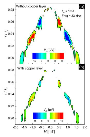
FIG. 7. (Color online) Contour plot of the magnetic field and temperature dependence of the measured dc voltage  $V_{\rm dc}$  with an ac current of 1 mA and frequency 33 kHz applied to sample Tr2b (a) without Cu layer and (b) covered with a Cu layer.
