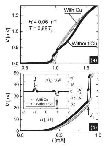
FIG. 6. (a) Voltage versus current for the sample Tr2b with and without a 500-nm-thick Cu layer on top. Panel (b) shows a low-voltage zoom-in of the panel (a) evidencing the same instability point  $J_1$  with and without Cu. The inset in panel (b) shows the rectified voltage  $V_{\rm dc}$  versus magnetic field when applying an alternative current of 1 mA and frequency of 33 kHz at  $T/T_c = 0.94$ .
