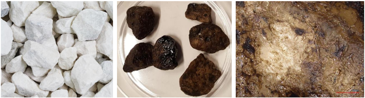
Figure. 1: the surface of a virgin marble aggregate (a), the same aggregate after the boiling water test (b) and a detailed surface scan after the boiling water test by confocal laser scanning microscope (c)
