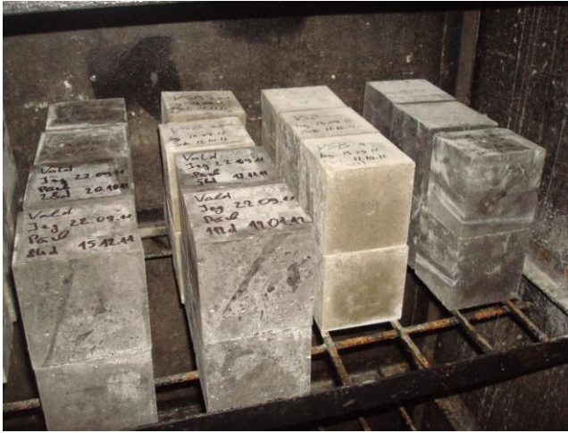
Fig. 1. Specimens with coal ash and wood ash substitution in curing chamber.
