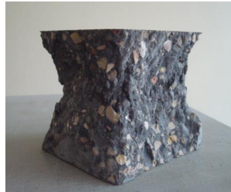
Fig. 3. Testing cube after compressive strength test has been carried out.
