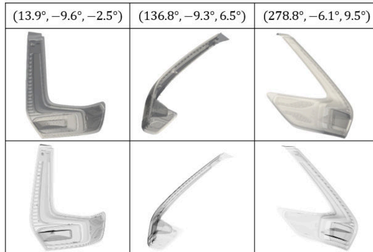
Figure 4: The CAD model of the object used in this study and the respective synthetic projections, created with the CAD projector, at the orientation (\gamma, \delta, \varphi) .
