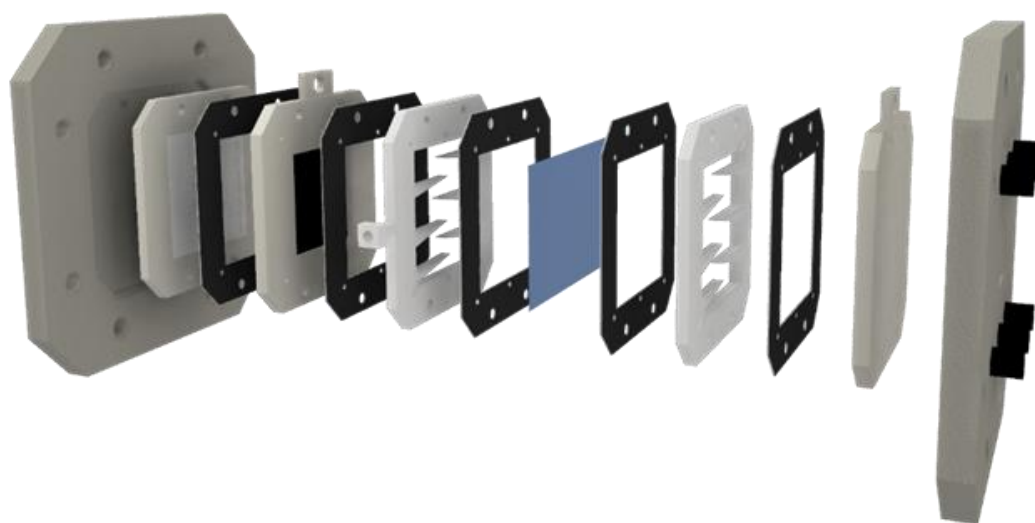
Figure 2. Detailed representation of the flow by reactor. Left to right: Aluminum back plate; Gas channel with turbulence promoter; Titanium cathode with GDE; Catholyte flow channel; Nafion® 117 membrane; Anolyte flow channel; Platinized titanium anode; Aluminum front plate with process connections; Rubber sealing.
