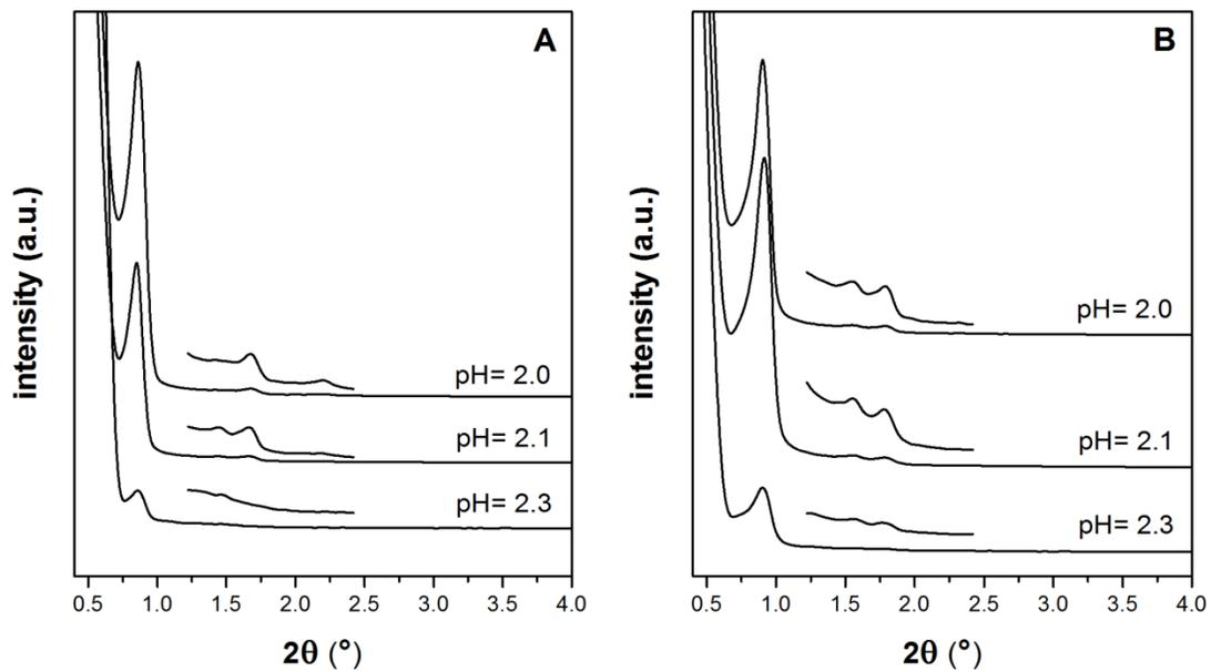
**Figure 6.** XRD patterns of ethane-bridged PMOs synthesized with the assistance of NaCl (PMO-11 to PMO-13 (Table 1)). A: as-synthesized samples, B: solvent-extracted samples
