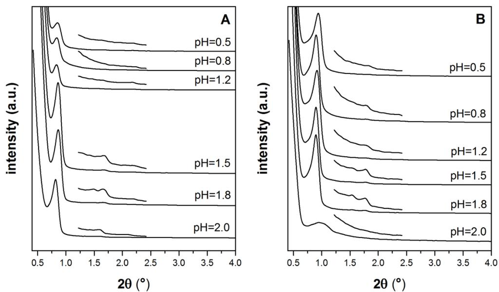
**Figure 1.** XRD patterns of ethane-bridged PMOs synthesized at different pH value ranging from 2.0 to 0.5 (PMO-2 to PMO-7 in Table 1). A: as-synthesized samples, B: solvent-extracted samples.
