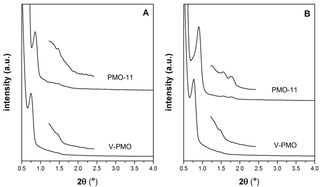
**Figure 9.** XRD patterns of PMO-11 and V-PMO synthesized at pH 2.3. A: as-synthesized samples
