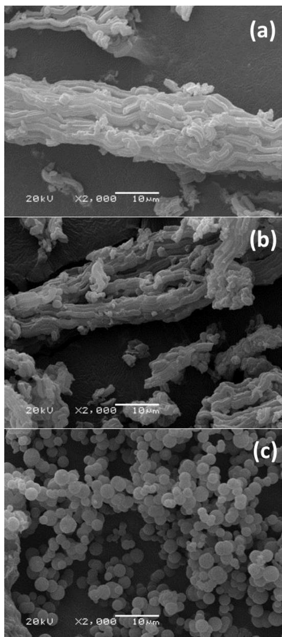
**Figure 8.** SEM images of ethane-bridged PMOs synthesized with the assistance of NaCl at different pH value: (a) pH=2.0 (PMO-13), (b) pH=2.1 (PMO-12) and (c) pH=2.3 (PMO-11).
