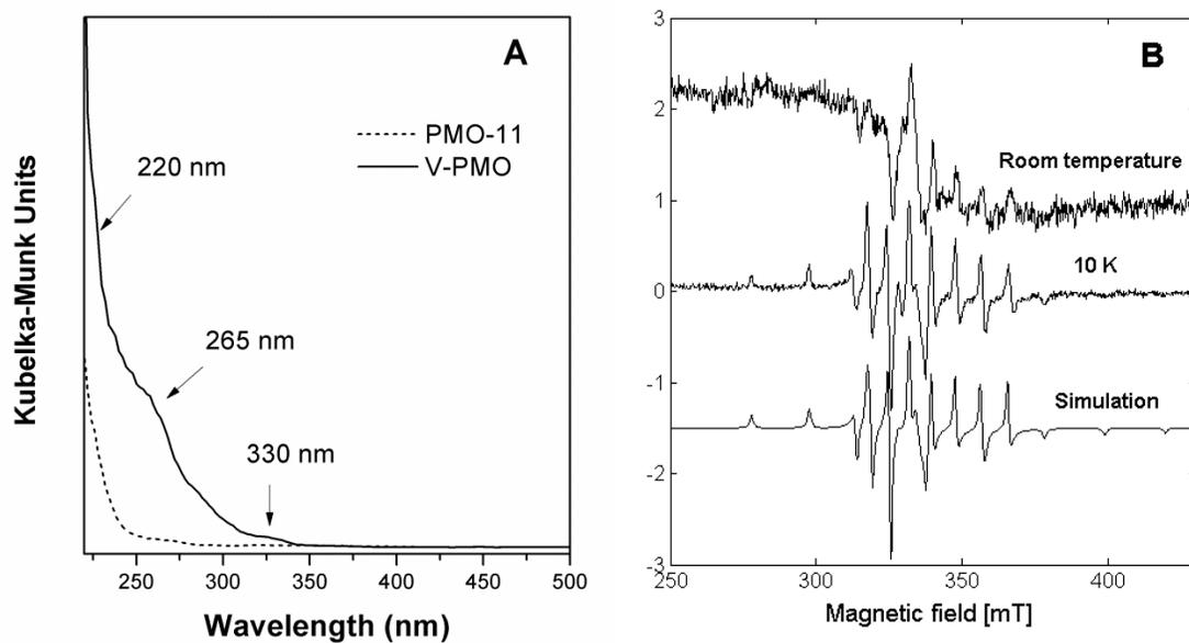
**Figure 10.** (A) DR-UV-Vis spectrum of PMO-11 compared to V-PMO. (B) CW-EPR spectra of solvent-extracted V-PMO recorded at room temperature and 10 K, respectively, and the simulated spectrum.
