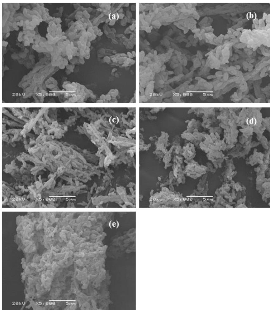
**Figure 3.** SEM images of solvent-extracted ethane-bridged PMOs synthesized at different pH value: (a) pH=1.8 (PMO-3), (b) pH=1.5 (PMO-4), (c) pH=1.2 (PMO-5), (d) pH=0.8 (PMO-6), (e) pH=0.5 (PMO-7).
