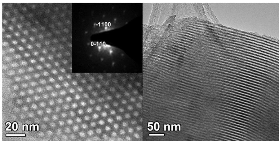
**Figure 4.** TEM images of solvent-extracted ethane-bridged PMOs synthesized at pH=1.8 (PMO-3) along different directions. The corresponding SAED pattern is presented as inset.
