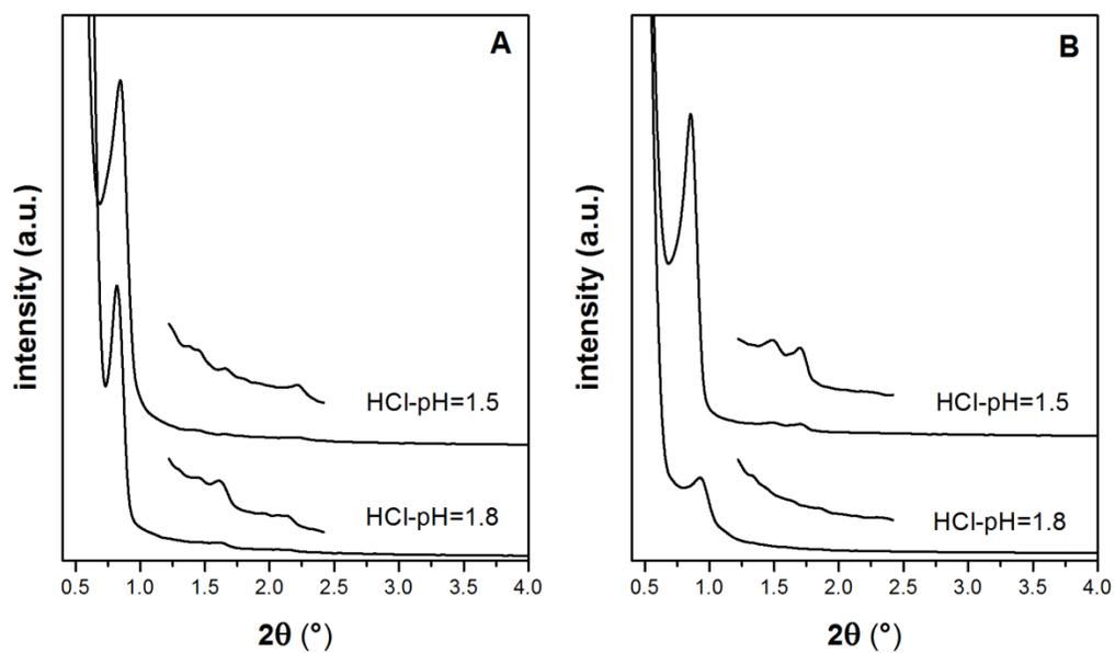
**Figure 5.** XRD patterns of ethane-bridged PMOs synthesized with HCl at pH=1.5 (PMO-10) and pH=1.8 (PMO-9). A: as-synthesized samples, B: solvent-extracted samples.
