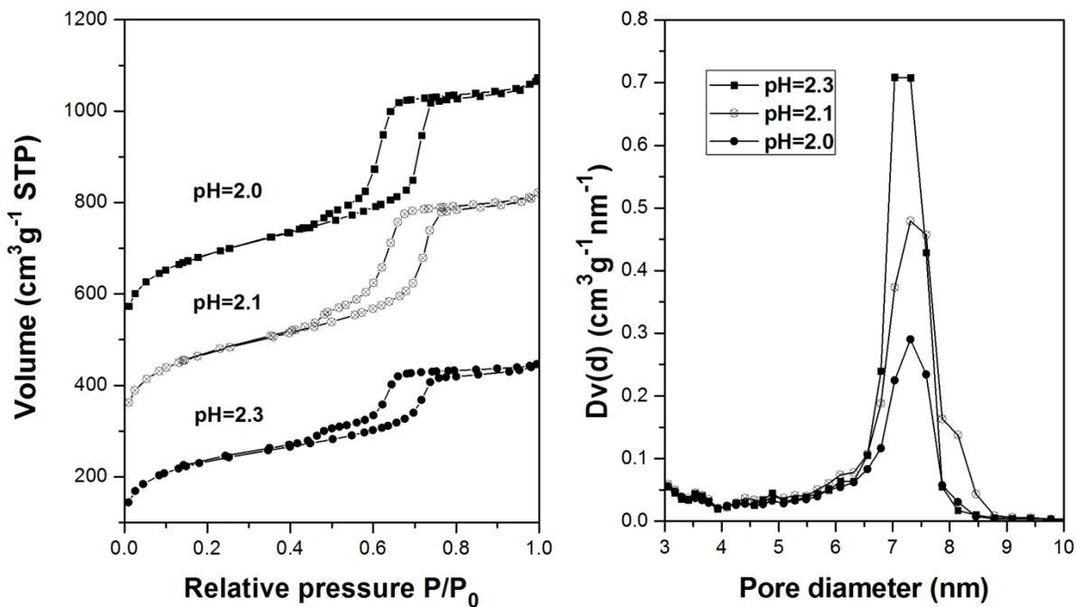
**Figure 7.** (left)  $N_2$  adsorption-desorption isotherms of ethane-bridged PMOs synthesized with the assistance of NaCl (PMO-11 to PMO-13 in Table 1), (right) corresponding pore-size distributions.
