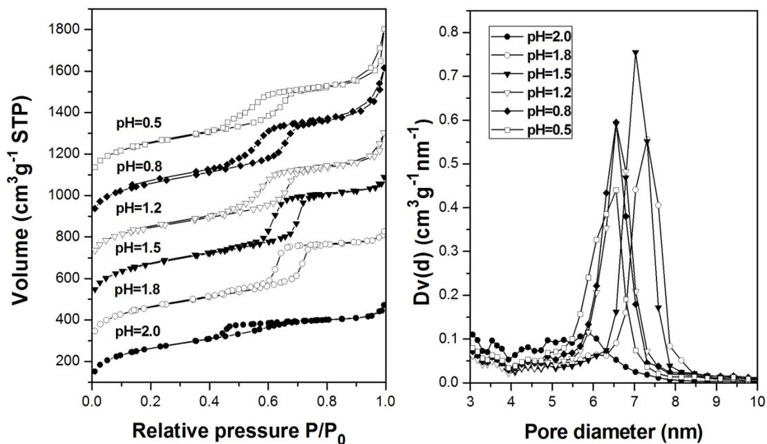
**Figure 2.** (left)  $N_2$  adsorption-desorption isotherms of ethane-bridged PMOs synthesized at different pH ranging from 2.0 to 0.5 (PMO-2 to PMO-7 in Table 1) and their corresponding pore size distributions, (right) corresponding pore-size distributions.
