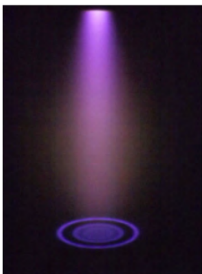
Figure 4. DC driven air glow discharge in a pin-water geometry with self-organization at the surface of the water anode electrode. Reproduced with permission from [56], copyright 2014 IOP Publishing.
