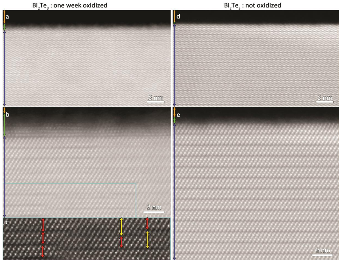
Figure 4.3 Cross-sectional overviews and close-up HAADF STEM images of the oxidized layers and the subsurface region of the one-week-oxidized \text{Bi}_2\text{Te}_3 (a, b) and the not explicitly oxidized \text{Bi}_2\text{Te}_3 (d,e). From top to bottom, a carbon protection layer (orange) is visible, followed by an amorphous layer intermixed with a distorted crystalline structure (green), and the \text{Bi}_2\text{Te}_3 structure (blue). The top part of the one-week-oxidized \text{Bi}_2\text{Te}_3 structure contains seven-layered defects (b,c), while the non-oxidized sample does not contain these defects (e). The areas in blue rectangles in (b) are enlarged with improved contrast in (c). (c) shows the stepwise displacement of the septuple layers (yellow arrows) in \text{Bi}_2\text{Te}_3 in the depth of the material, which is in agreement with the model of Jiang et al. 250 . The quintuple layers are marked with red arrows.
