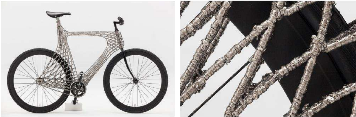
Figure 2. The 3d-printed bicycle (left) and the joints close-up (right)
