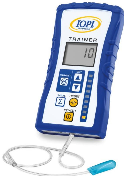
Fig. 1 Iowa Oral Performance Instrument (model 3.2, IOPI Medical LLC, Woodinville, WA, USA)
