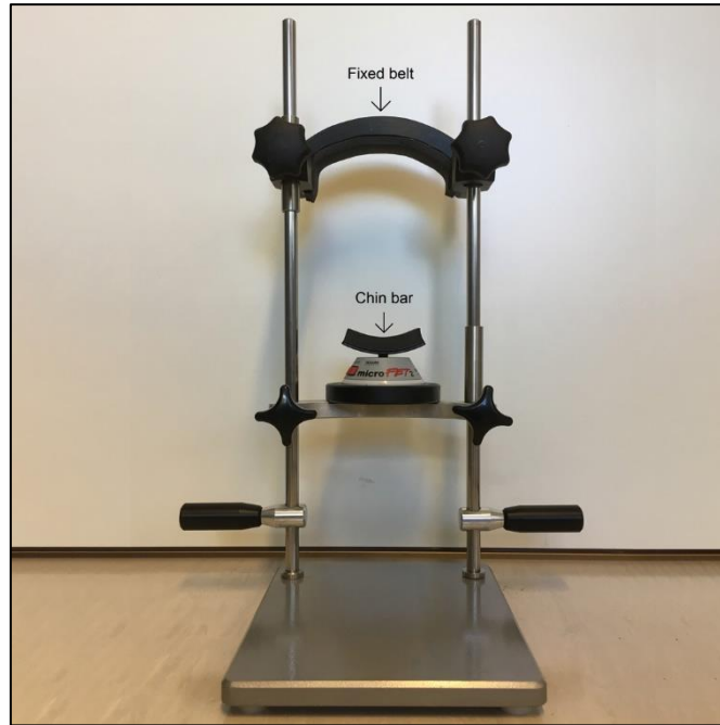
Fig. 2 Examination frame and dynamometer (Microfet™, Biometrics, Almere, The Netherlands)
