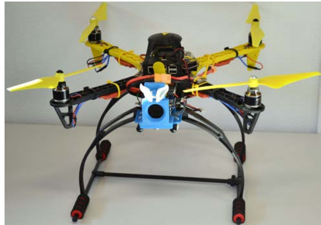
Fig. 8. Image showing an ERLE-COPTER drone with a Raspberry Pi as its main processor unit. In the front, our sonar sensor platform easily fits on the enclosure. Since this drone should support payloads up to 1 kg, according to the documentation, it should be feasible to generate enough lift to fly with our sonar sensor platform, which weighs only 90 g, mounted on it.
