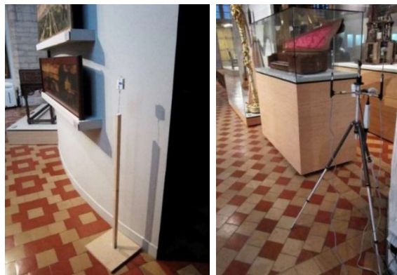
Figure 6.1.1 a (left) and b (right); Hobo U 12 data logger during the installation (left); Innova MM 0036, MM 038, MM 060 and Vaisala GM 70 sensors during the installation
