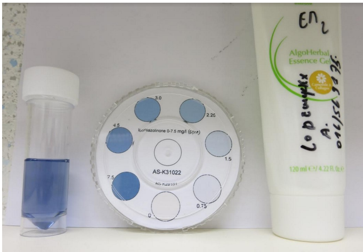
Fig. 2 Experimental spot test indicating the potential presence of isothiazolinones in the facial gel mask.
