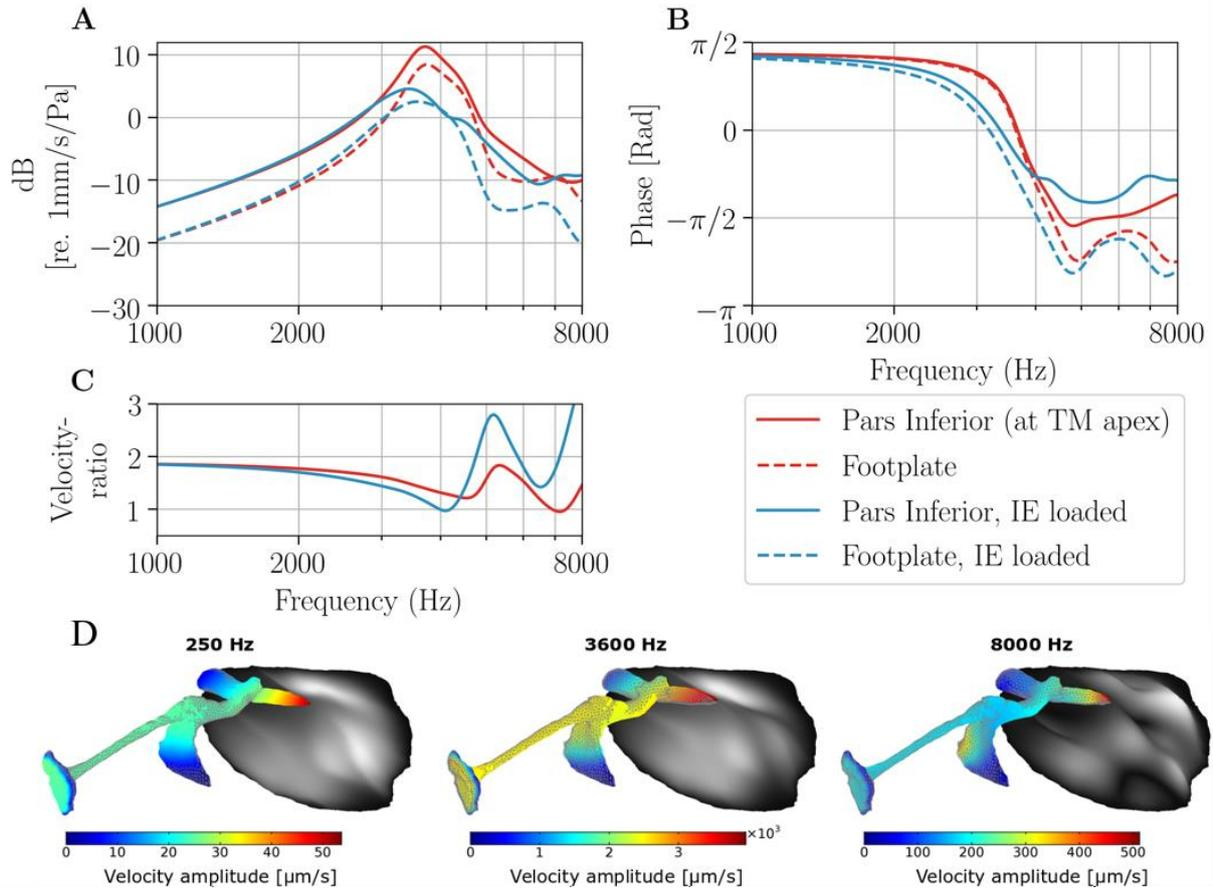
288 **Figure 3.** PI and FP response of the loaded and unloaded ME system with the material parameter values of Table 1. (A) velocity
