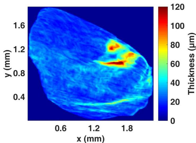
158 **Figure 2.** Thickness distribution of the TM of the anole. The thickness is largest where the PI attaches to the TM. The average
