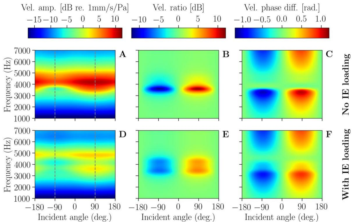
355 **Figure 5.** Results of the internally coupled ME model with (top row) and without (bottom row) IE loading. (A) IL TM vibration
