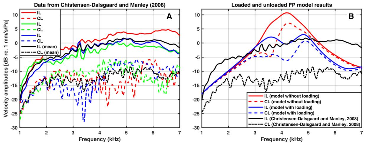
351 **Figure 4.** (A) Measured individual and averaged transfer functions of the ipsilateral (IL) and contralateral (CL) TM normalized
