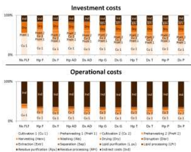
Fig. 6 Contribution analysis of the different process steps to the investment and operational costs of all Pareto-optimal scenarios
