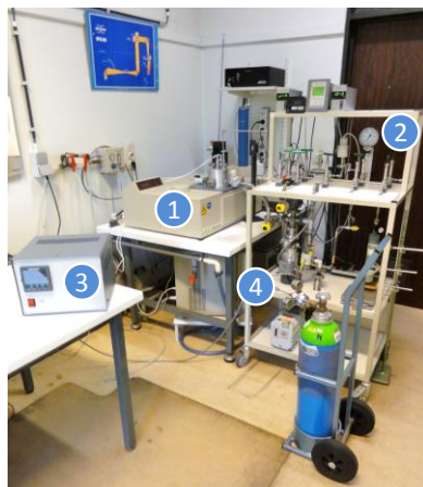
Figure 2.3: Overview of the used experimental FTIR setup: (1) Bruker 66v FTIR vacuum spectrometer, (2) vacuum manifold, (3) PID controller and (4) two-stage pump group.
