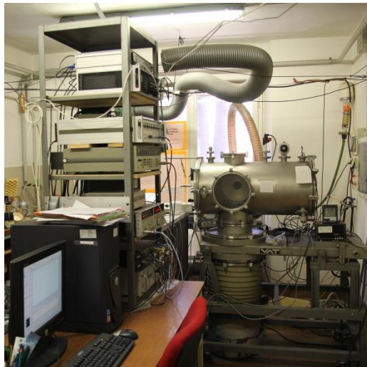
Figure 2.7: Photograph of the Balle-Flygare type FTMW spectrometer used at the University of Bologna, with the controllers and amplifiers on the left-hand side and the Fabry-Pérot cavity on the right.
