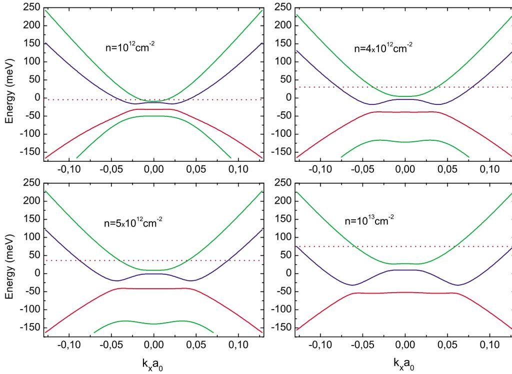
FIG. 9. (Color online) The band structure of the four-layer graphene with the full interaction as a function of  $k_x$  (around the  $K$  point for  $k_y=0$ ) for different values of the total density (the horizontal dotted line corresponds to the Fermi energy).
