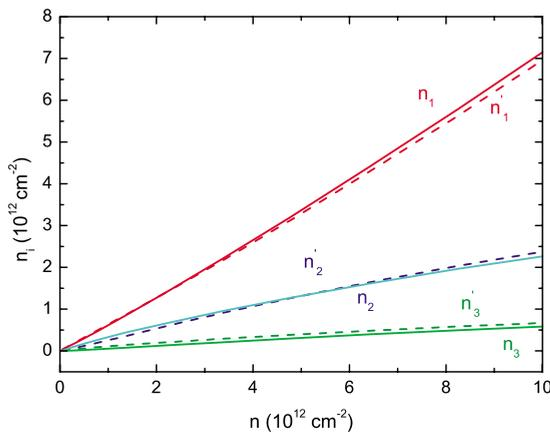
FIG. 7. (Color online) The layer densities  $n_i$  (solid curves) for the three-layer system with the full interaction and  $n'_i$  (dashed curves) for the case when only  $\gamma_0$  and  $\gamma_1$  are different from zero, as a function of total excess density  $n$ .
