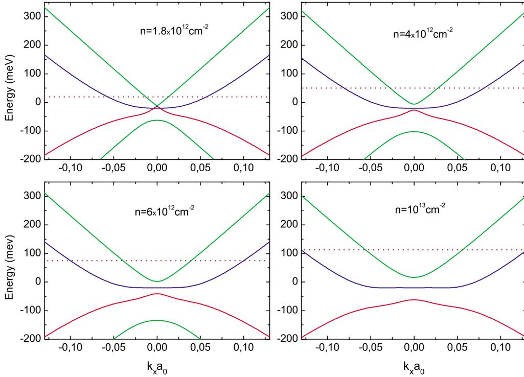
FIG. 6. (Color online) The band structure of the three-layer graphene with the full interaction as a function of  $k_x$  (around the  $K$  point for  $k_y=0$ ) for different values of the total density. The horizontal dotted line corresponds to the Fermi energy.
