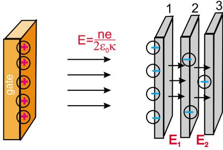
FIG. 1. (Color online) Schematic of the three-layer graphene system near a positively charged gate, which induces a total excess density  $n=n_1+n_2+n_3$ , with  $n_1$  the excess density of electrons on the closest layer to the gate, and  $n_2(n_3)$  is the excess density on the second (third) layer;  $E_i$  ( $i=1,2$ ) is the uniform electric field between the layers with  $E_1=(n_2+n_3)e/\epsilon_0\kappa$  and  $E_2=(n_3)e/\epsilon_0\kappa$ .
