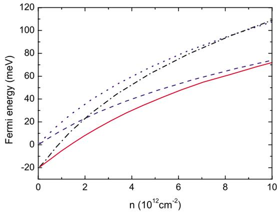
FIG. 3. (Color online) The dependence of the Fermi energy  $\varepsilon_F$  on the total density  $n$  for three-layer graphene in the case when we neglect all interactions except  $\gamma_0$  and  $\gamma_1$  (dotted curve) and include all interactions (dotted-dashed curve). The dependence for  $\varepsilon_F$  for the four-layer graphene when we neglect all interactions except  $\gamma_0$  and  $\gamma_1$  (dashed curve) and for the full interaction case (solid curve).
