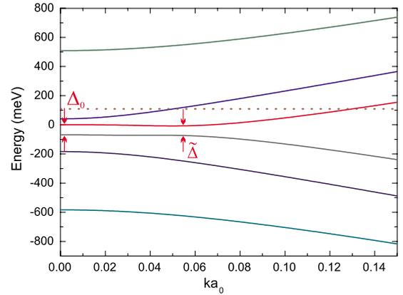
FIG. 2. (Color online) The band structure of three-layer graphene around the  $K$  point for a total excess electron density  $n=10^{13}$   $\text{cm}^{-2}$  in the case when we neglect all interactions except  $\gamma_0$  and  $\gamma_1$ . Horizontal dotted line is the Fermi level.
