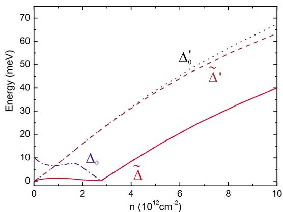
FIG. 4. (Color online) The dependence of the gap  $\Delta_0$  at the  $K$  point (dotted-dashed curve) and the true gap  $\tilde{\Delta}$  (solid curve) for three-layer graphene when including the full interaction as a function of the total excess electron density  $n$ . For comparison we show also the corresponding results,  $\Delta_0'$  (dotted curve) and  $\tilde{\Delta}'$  (dashed curve), when only  $\gamma_0$  and  $\gamma_1 \neq 0$ .
