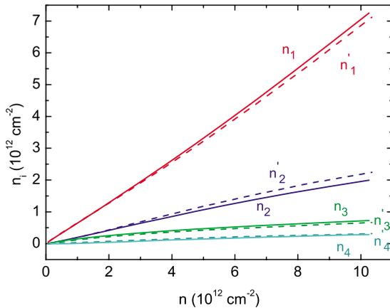
FIG. 10. (Color online) The layer densities  $n_i$  (solid curves) for the four-layer graphene with the full interaction and  $n'_i$  (dashed curves) for the case when only  $\gamma_0$  and  $\gamma_1 \neq 0$  as a function of total excess density  $n$ .
