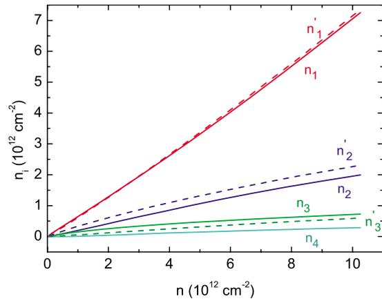
FIG. 11. (Color online) The layer densities  $n_i$  for the four- (solid curves) and  $n'_i$  (dashed curves) for three-layer graphene systems respectively, as a function of total excess density  $n$  (for the full interaction case).
