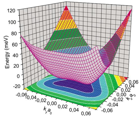
FIG. 5. (Color online) The first conductivity band and the contour plot for three-layer graphene with the full interaction included around the  $K$  point for a total excess electron density  $n = 1.5 \times 10^{12} \text{ cm}^{-2}$ .
