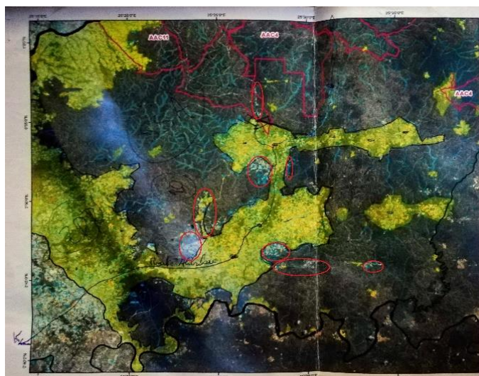
Figure 4. Landsat 8 satellite map of a part of ITC's concession, from 10/05/2017. The mapped RDZ was reshaped as it extended outside of its foreseen boundaries (we highlighted some of these extensions by red circles).
