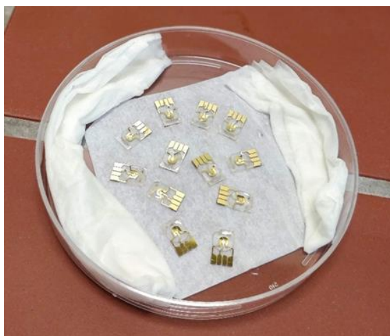
Figure 2.2 Microelectrodes kept in humid conditions with wet tissue papers in the vicinity and sealed for overnight immobilization of ssDNA through chemisorption.
