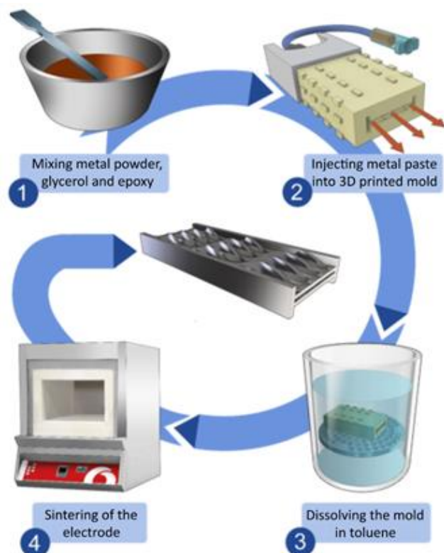
Figure 1. Indirect 3D printing method
