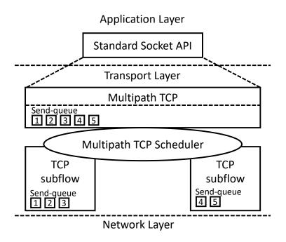
Figure 7: The Multipath Transmission Control Protocol (MPTCP) architecture [81].
