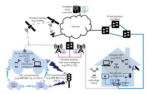
Figure 1: Representation of a subset of different heterogeneous networks and their interconnections
