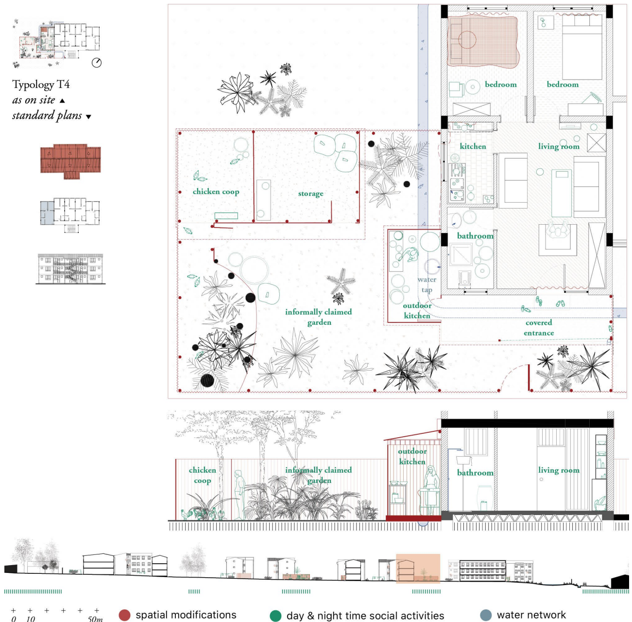
Fig 3. Housing typology with spatial modifications (red), social activities (green) and water network (blue). Structural and non-structural spatial modifications were mapped in red. They comprise informal housing extensions, added doors, removed walls, elevations and adjustments to the windows and other potential mosquito entry points. Spatial mosquito protective measures such as bed nets, curtains and other coverings of holes for screening purposes were also indicated in red, and complemented with socio-cultural activities and practices taking place at day (light green) and night times (dark green), such as cooking or laundering. These observations form a layer of appropriation of either the condominiums common spaces or the standardized housing plan. Finally, a blue layer was added to highlight the water network, including rivers, meanders, canals, and water taps.
