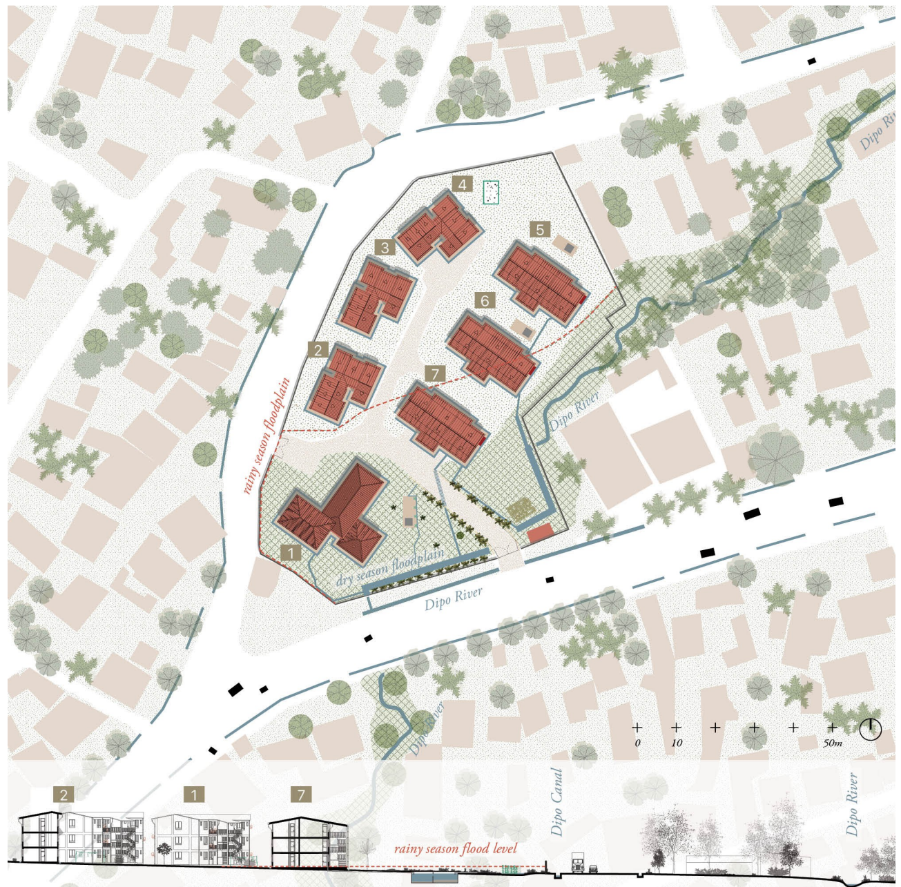
Fig 6. Disruptive water networks in Condominium D. Condominium D is located in the Dipo River floodplain, flooding the site moderately in dry season and extensively in rainy season (red dotted line). Within the walls of the condominium, the river is canalised and used as outlet for both the rain gutter network coming from the housing blocks and the septic tanks. The site suffers from permanently stagnating water. Map drawn by the authors, based on https://www.usgs.gov/ and openstreetmap.org .
