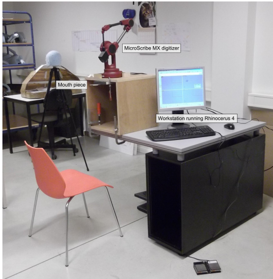
Figure 8: Experiment setup. The test subject was seated on the red chair, biting down on the white mouth piece to stabilize their head. The box fixating the MicroScribe was positioned such that the experimenter could comfortably move the digitizer’s arm around the person’s head.
