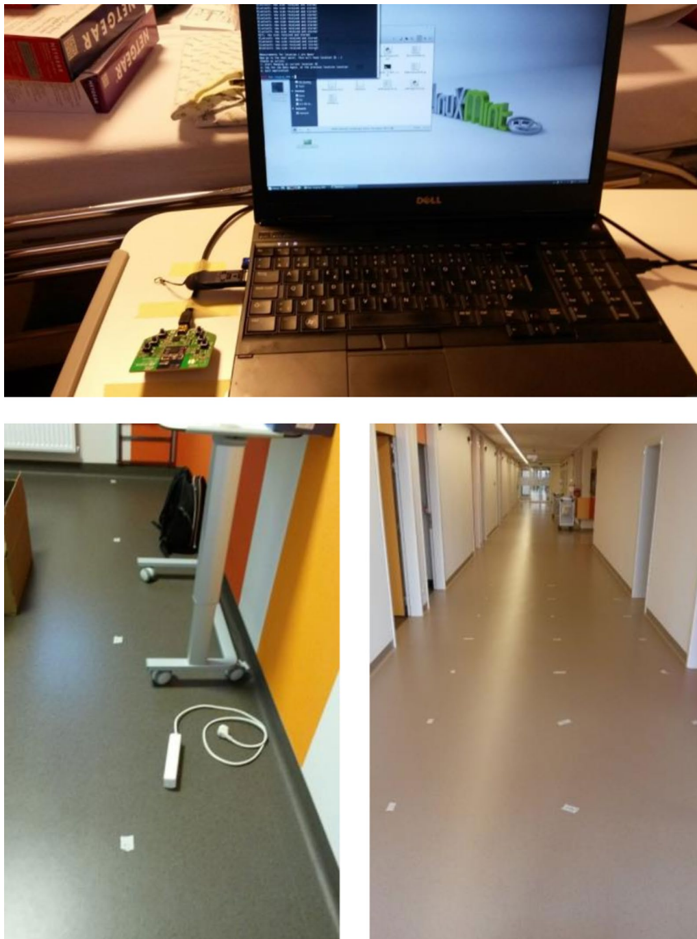
Fig. 6 The mobile node: a Dell laptop with 3 dongles (Wi-Fi, BLE, sensor node STM32) at a trolley at 100 cm height. The ground truth of the evaluation points was indicated on the white sticker on the floor resulting in a grid of 1 m by 1 m. Picture of a room and the corridor
