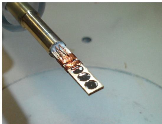
FIG. 1. C2 electric contact aperture holder mounted with a solenoid. Extreme left and right contacts power the solenoid.
