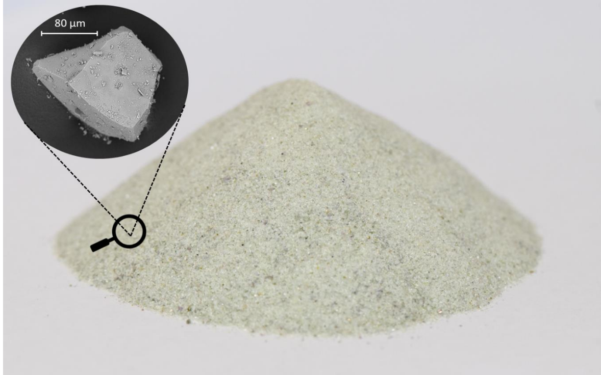
Figure 1.4: Picture of the experimental Norwegian dunite sand (93 – 332 \mu\text{m} ) and a detailed scanning electron microscope image of a singular olivine grain that is covered with fine (<10 \mu\text{m} ) olivine particles originating from the industrial grinding process.
