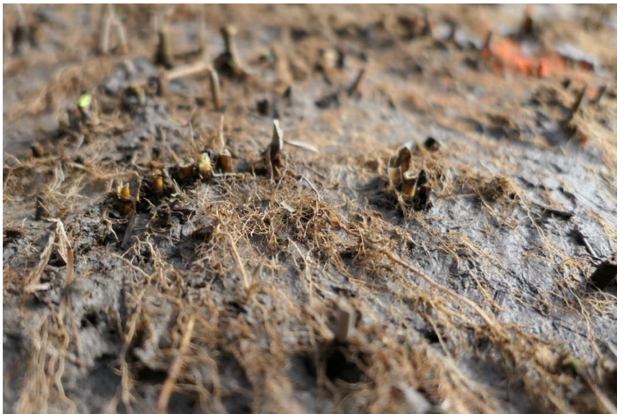
Figure 6.7: Sediment surface after the last experimental run with the emerging shallow subsurface mat of fine roots. Note that above-ground shoots have been manually clipped.
