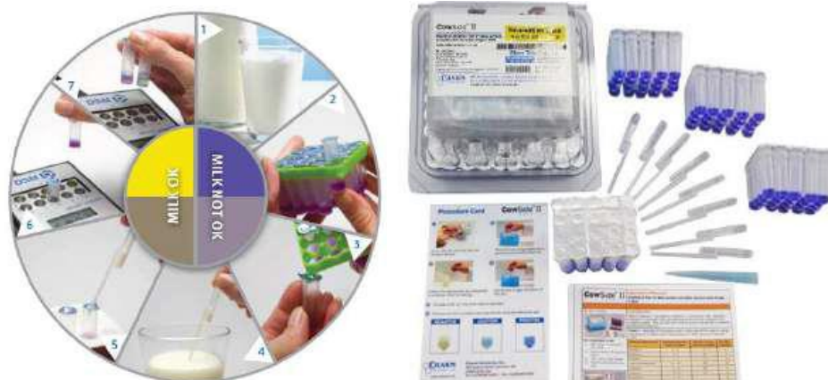
Fig. 1.4 Example of microbial inhibition tests, commercially known as Delvotest and CowSide II On the left: the main steps needed to perform a Delvotest. On the right: the complete kit of CowSide II (from company websites).
