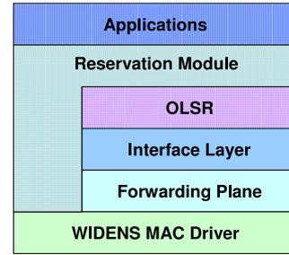
Fig. 1. Main components of the network layer of a WIDENS node
