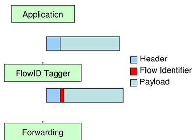
Fig. 3. Adding a flow identifier into data packets
