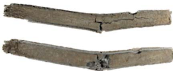
Obr. 7. Litera s prasklinami [2] Fig. 7. A letter with cracks [2]
